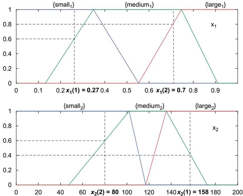
Fig. 1. A full fuzzy covering (discretization) with three fuzzy sets with 50% overlap on two attributes  $x_1$  and  $x_2$ , respectively.
