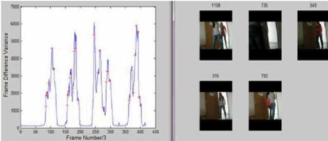
Figure 4. Frame difference variance curve and corresponding key frames without illumination intensity change.
