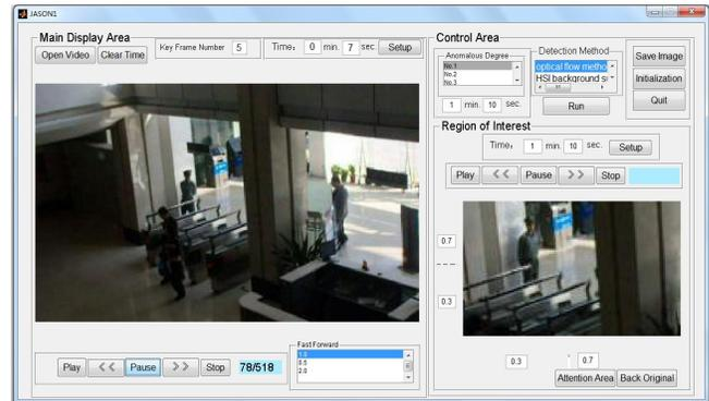
Figure 3. User interface of moving object detection system. The left-hand window is the Main Display Area, the upper-right window with parameter settings is the Control Area and the bottom-right window is the Region of Interest selected from the main scene by users through interactive tools.
