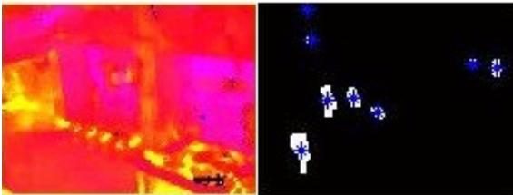
Figure 9. Generated three-channel composite image and connected domains by HSV background subtraction method.
