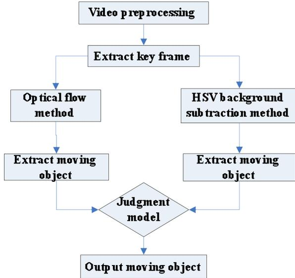
Figure 2. Hybrid moving object detection system flowchart.
